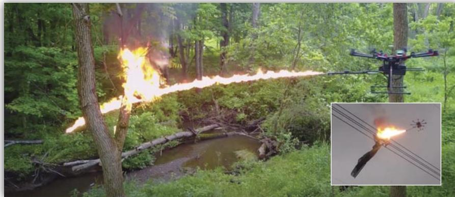
TF-19 WASP Flamethrower Drone shown here removing a kite from power lines and a large wasp nest near a hiking trail.
